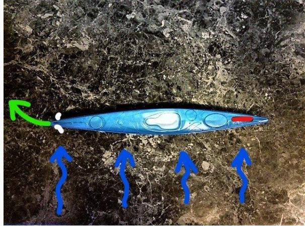
Another common question I hear is: “My skeg is down and the boat still turns, why?!” Notice the bow wake is much smaller because the paddler has slowed their pace, which decreases the pressure of the wake holding the bow in place. Since the skeg is still deployed, it is now locking the stern in tighter than the bow, causing the kayak to turn away from the wind.
