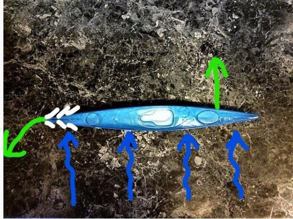
In this photo, the paddler is taking forward strokes and has the boat at the average paddling speed of 3 knots. The wind is still blowing against the side of the boat, which is causing their kayak to turn into the wind, this is called weather-cocking.
