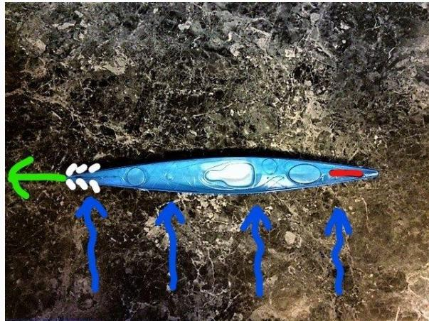
Here in photo 3, to stop the boat from turning into the wind, the paddler has lowered the skeg. By lowering the skeg, the stern of the boat locks in and does not let the wind blow it sideways. Now, the kayak has restored even pressure against the wind and the boat straightens out.
