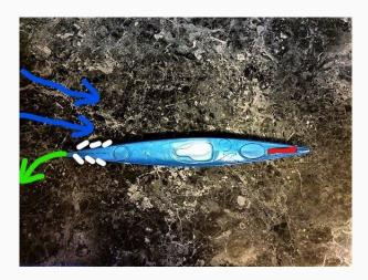
When paddling into the wind with the skeg down, it's hard to stay on course. The boat wants to turn sideways in relation to the wind because it wants to even out the bow and stern pressure(see picture 3), which causes it to turn away from the wind making it very difficult or impossible to stay on course.
