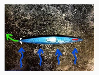
Another common question I hear is: "My skeg is down and the boat still turns, why?!" Notice the bow wake is much smaller because the paddler has slowed their pace, which decreases the pressure of the wake holding the bow in place. Since the skeg is still deployed, it is now locking the stern in tighter than the bow, causing the kayak to turn away from the wind.
