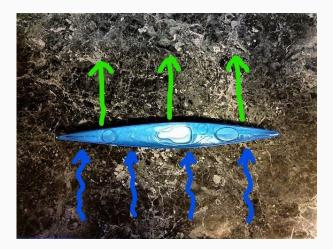
Here, the boat is at rest and the paddler is not taking any strokes. The wind is blowing against the side of the boat (depicted by the blue lines). In this scenario, the kayak orients itself so it has even pressure from the wind down the entire side causing it to blow across the water sideways.
