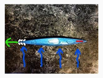
Here in photo 3, to stop the boat from turning into the wind, the paddler has lowered the skeg. By lowering the skeg, the stern of the boat locks in and does not let the wind blow it sideways. Now, the kayak has restored even pressure against the wind and the boat straightens out.
