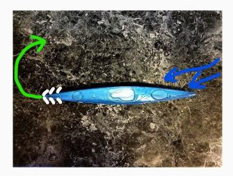
Once the skeg is raised, the wind will push the stern around causing the boat to turn into the wind.
